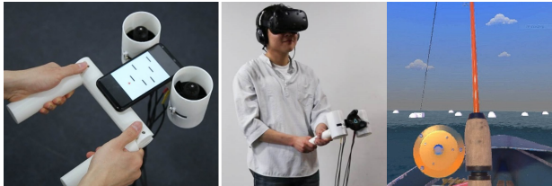
Figure 16. Flight control application & Fishing application: Device is attached to a small display running an airplane game, giving the user tilt feedback corresponding to the game (left). User shown holding the device with a fishing rod handle shaped attachment and wearing a HMD (middle). User's point-of-view within the fishing application (right).
