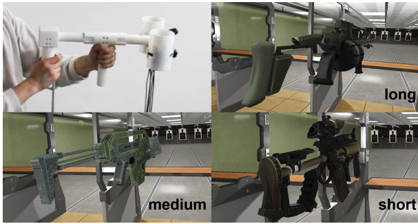
Figure 15. Gun VR application: User shown holding the device with a gun handle shaped attachment and wearing a HMD (top left). Different haptic feedback is given to the user corresponding to the length of the gun, and muzzle rise feedback is given while the trigger is pressed.
