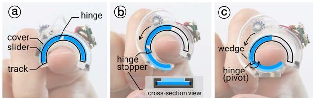
Figure 7: The key to our mechanism's unfolding is that (a) its cover is comprised of two segments; (b) our hinge is based on two detents that create a stopper and (c) force the cover to pivot and be pushed by the wedge against the fingerpad.
