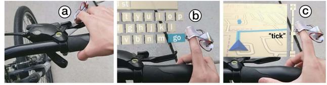
Figure 5: (a) User grips the bike handle while wearing our device. (b) As they type the address, our device renders the clicking of the keys. (c) When they drag the slider, our device renders haptic detents that depict the magnification levels.
