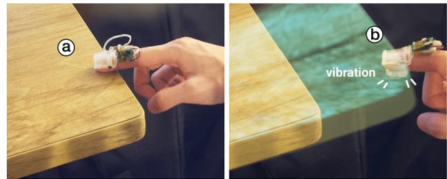
Figure 12: In our interior design application, (a) users can feel both the real table but also, (b) the virtually-extended table.
