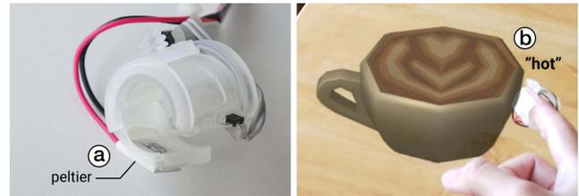
**Figure 21:** Example of integrating a Peltier element onto our foldable actuator: (a) The Peltier element attached to the cover; and, (b) as the user touches the virtual coffee cup they feel not only contact but also actual heat.
