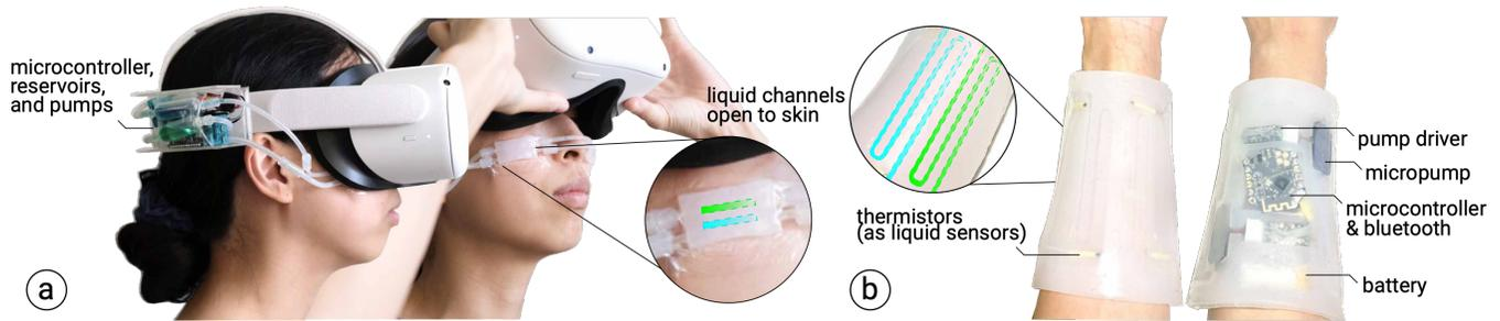
**Figure 7:** We designed two versions of our device to deliver liquid stimulants to two locations – the cheeks and the arm. These also showcase two engineered solutions for delivering our chemicals to the skin: (a) a central control & pump unit connected to silicone patch via tubing or (b) fully encased and self-contained silicone wearable, including microcontroller, pumps, and battery.
