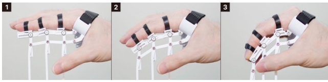
Figure 5: The pin slots successfully absorb the distance displacement of the inner joints and transmit finger motion.
