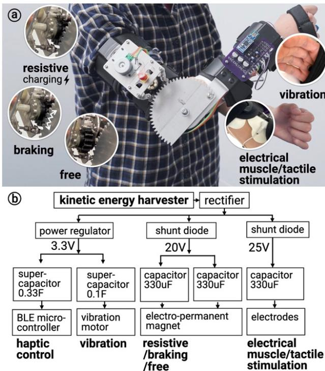
Figure 14: (a) The various available haptic output provided by our device. (b) Diagrammatic view of each sub-capacitor/supercapacitor depending on its haptic output.
