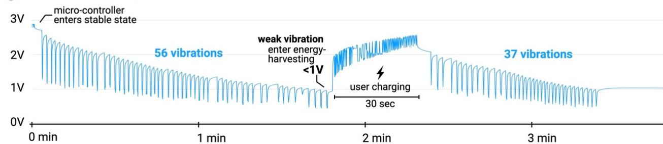
Figure 16: (a) Charging and discharging profile of our 0.33F supercapacitor used to power the haptic device’s microcontroller. (b) Charge/discharge profile of the two capacitors that switch our haptic device’s EPM clutch and the braking mode. (c) Charge/discharge profile of the capacitor used for electrical muscle stimulation, of 300ms in duration. (d) Charge/discharge profile of the super-capacitor used for vibrations, of 300ms in duration.
