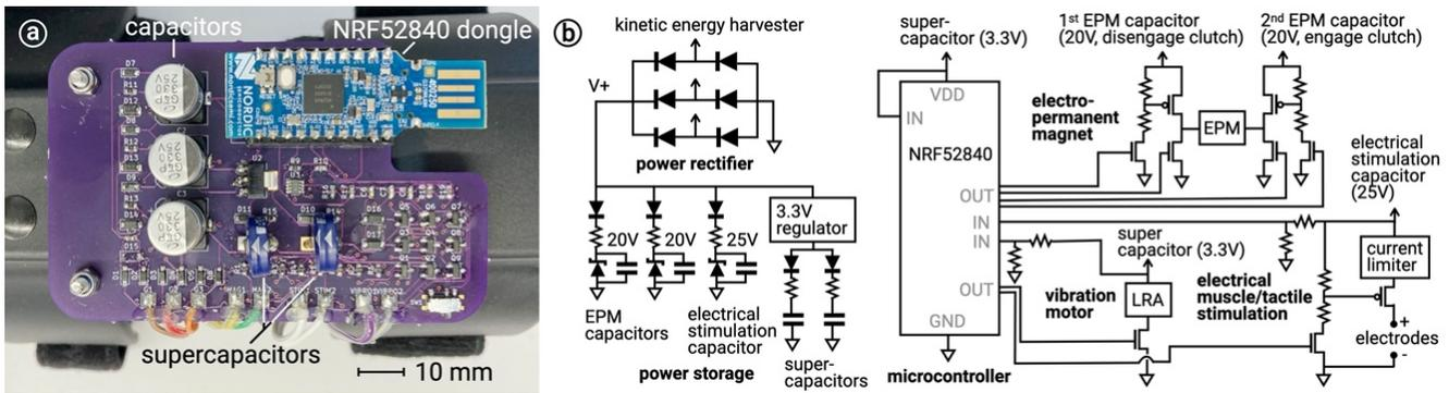
Figure 13: (a) Our custom PCB containing energy harvesting and haptic control circuits. (b) Schematics of our PCB, V+ depicts the DC power which can range from 0-35V when charged by the arm, regulated into sub-voltages for the microcontroller and actuators.
