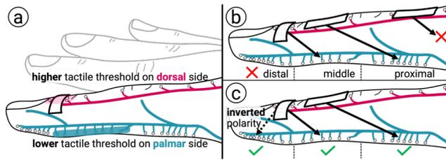
**Figure 3: (a) Tactile threshold for electrical stimulation is significantly lower on the palmar side than on the dorsal side. (b, c) Utilizing both polarities (anodic and cathodic) for the electrode attached to the fingertip enables stimulation of the fingerpad.**
