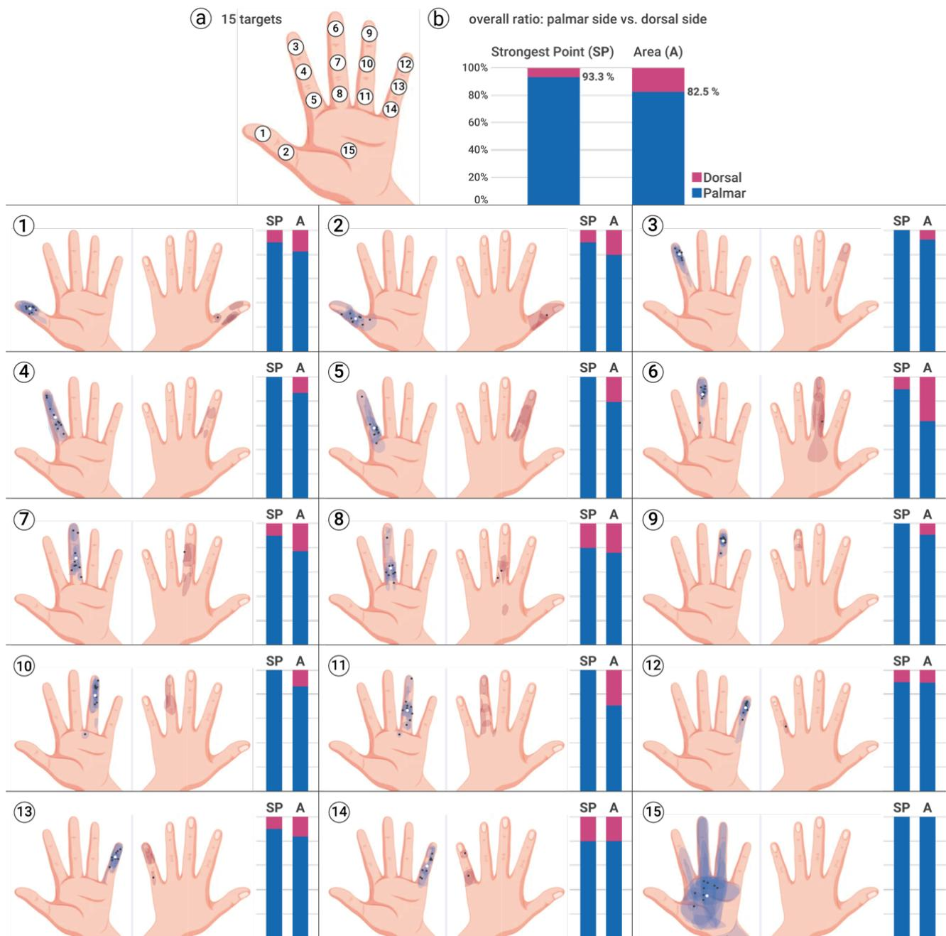
**Figure 7: (a) The 15 target locations on the palmar side of the hand to elicit tactile sensation via our back-of-hand electro-tactile stimulation. (b) The overall ratio of the tactile sensation elicited on the palmar vs. dorsal side. (1-15) Overlaid raw data for all participants; black points correspond to strongest points; white points are averages; colored shades depict the area indication.**
