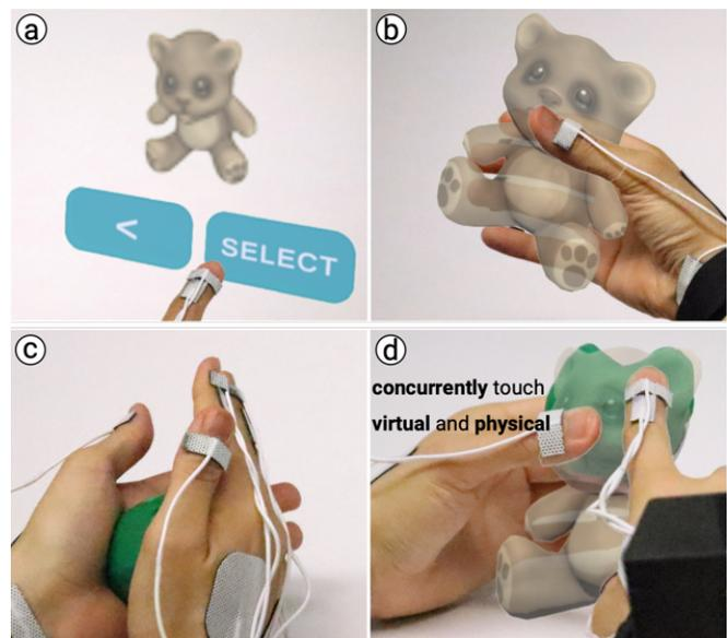
Figure 11: MR clay application alongside virtual 3D models (superimposed the virtual content for the sake of visual clarity).
