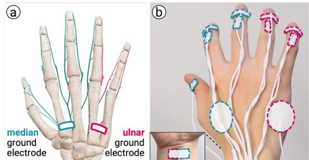
**Figure 4: We implemented (a) two ground electrodes to avoid median/ulnar interference. (b) Our final electrode arrangement.**
