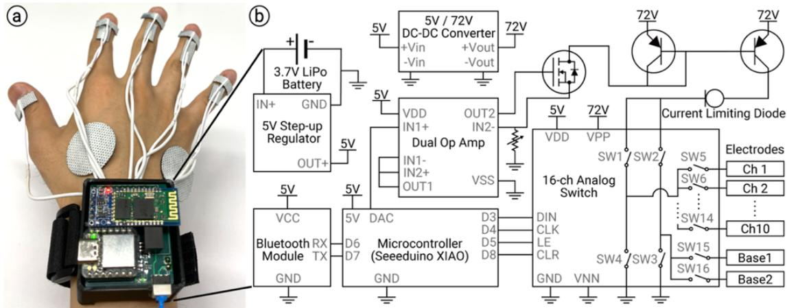
Figure 5: (a) Out wrist-worn electro-tactile stimulator. (b) Electronics schematics of our custom electrical stimulator.
