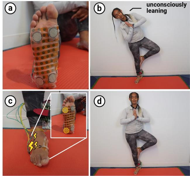
Figure 14: Postural control via electrotactile while barefoot.
