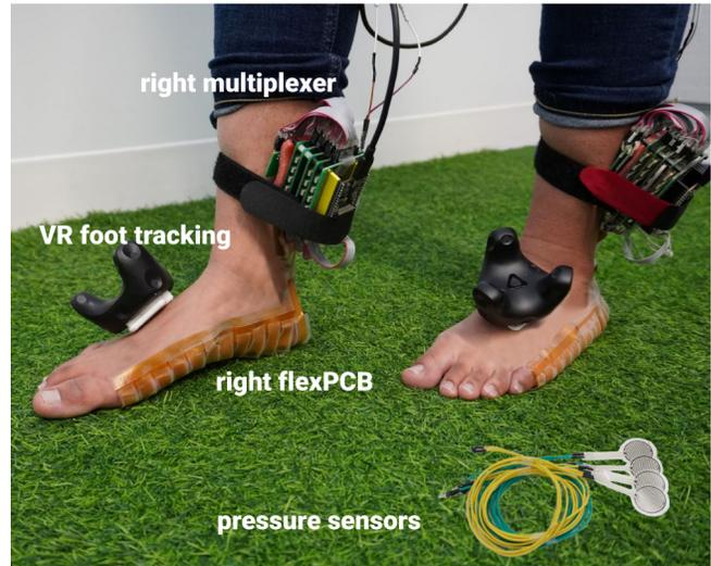
Figure 6: Key hardware attached to the user’s feet: one of flexPCB with 60 electrodes for each foot, a multiplexer unit for each electrode array, tracking for any VR application, and four pressure sensors (FSR) worn at the sole for balance detection.
