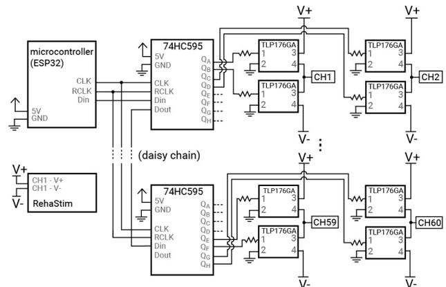
Figure 3: Our multiplexer circuit for 60 channels.
