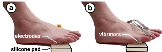
Figure 8: The study setup. Participants stand on the (a) electrodes or (b) vibrators and a silicone pad.
