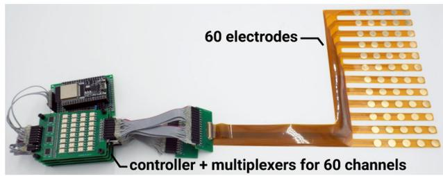
Figure 2: A prototype of electrodes and stimulation devices.
