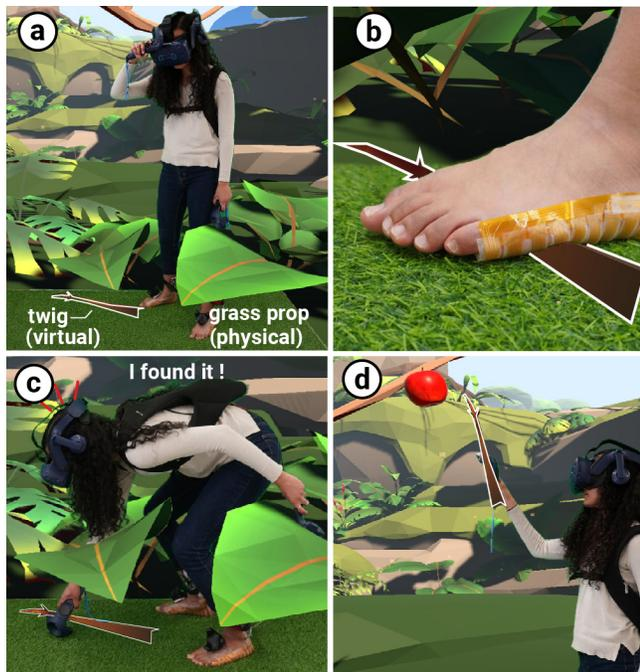
Figure 13: Using FeetThrough to feel both virtual sensations from stepping on VR objects as well as real ground props.
