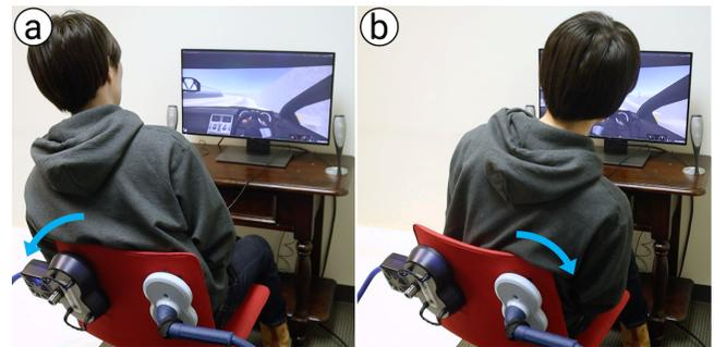
Figure 10. Muscle actuation through the fabric of the chair. As the car turns (a) left or (b) right, users feel force-feedback.
