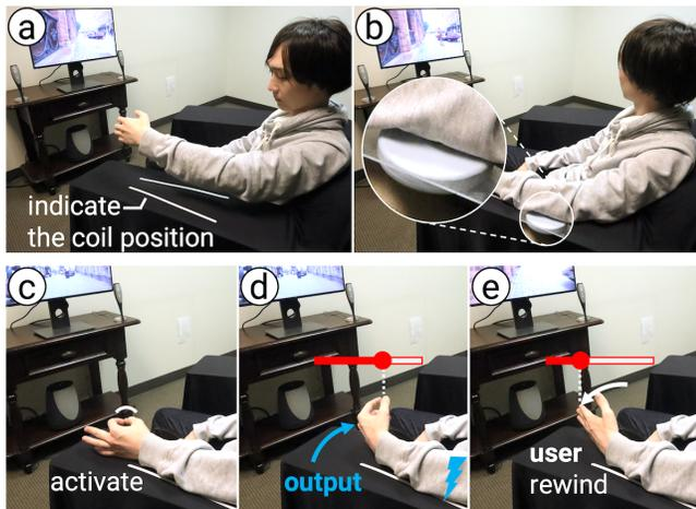
Figure 8. Our video-scrubbing tool based on MMS can extend EMS-based I/O interaction by improving the clarity of its output and installing the system into the furniture piece.
