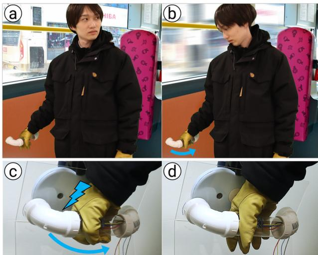
Figure 9. (a, b) Envisionment of MMS in a bus handle where its handle automatically actuates the passenger's grab when the
