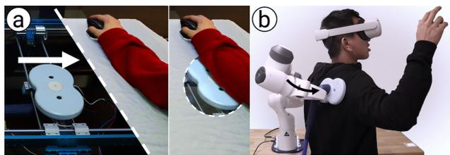
**Figure 13.** An alternative to strategic coil placement is to motorize the coil, e.g., using (a) X-Y gantry or (b) robotic arm.
