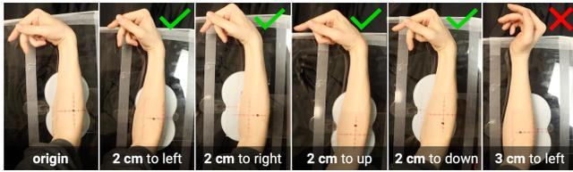
**Figure 12.** An example and measurement of how deviation in coil alignment could impact the resulting wrist movements.
