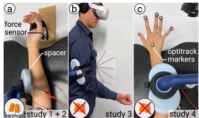
**Figure 3.** Overview of our study setups. In Study#1, we had an additional spacer to adjust the coil distance (e.g., 20 mm), and the EMS electrodes were not present as this study focused solely on MMS. In all EMS conditions, we used 1.5-inch pre-gelled electrodes and biphasic stimulation, a method commonly employed in previous work (e.g., [42]), to mitigate skin tingling.
