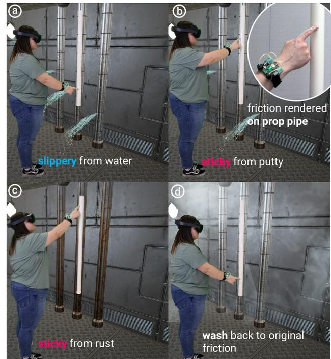
**Figure 15: Stick&Slip adds friction feedback to VR with props.**
