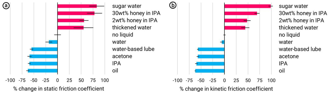
Figure 9: Relative changes in: (a) static friction, and (b) kinetic friction for each fluid.
