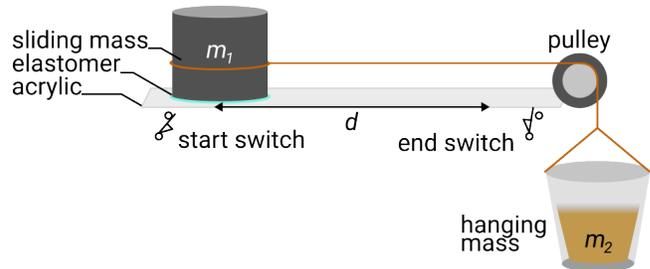
**Figure 8: We built a mass-pulley tribometer to mechanically evaluate the effect of our liquids on coefficient of friction.**
