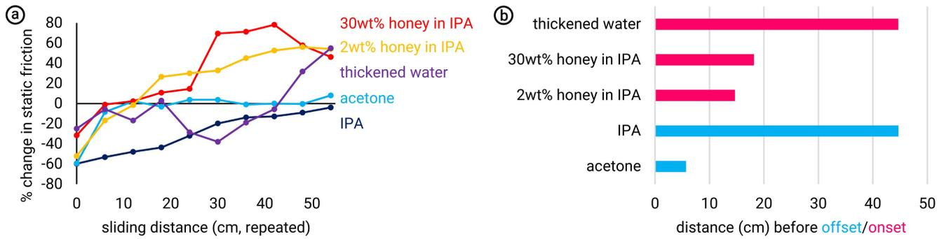
**Figure 11: (a) Fluid friction over repeated trials (distance in cm); and (b) offset/onset distance (i.e., the sliding distance required for a slippery sensation to disappear or a sticky sensation to appear).**
