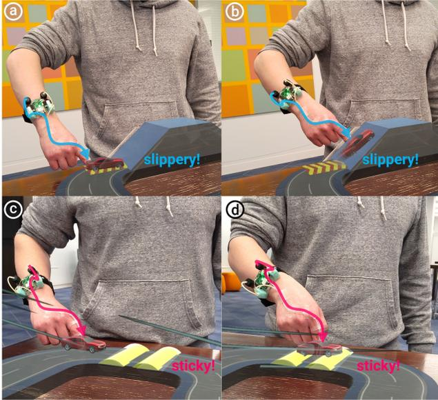
Figure 6: Our device alters the friction of everyday objects, such as on top of this toy ramp or speedbumps.
