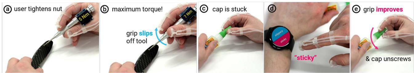
**Figure 16: Stick&Slip with tools:** (a) A user tightens a nut via a digital torque screwdriver. (b) At the maximum torque, our device pumps slippery liquid to provide an additional haptic cue. (c) A user unsuccessfully tries to open their glue. (d) The user activates on-demand stickiness, which increases friction and improves grip, (e) which assists the user to unscrew the cap.
