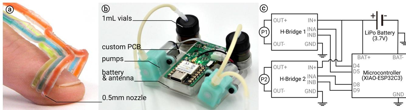
Figure 7: (a) Our nail-worn droplet generator. (b) Our bracelet device and its components. (c) Electronics schematic of our PCB.
