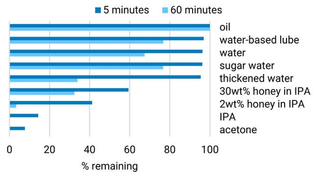
Figure 10: Fluid evaporation at two points (5 and 60 minutes).
