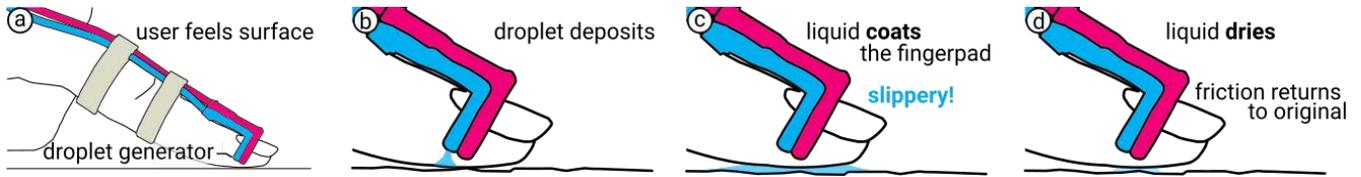
**Figure 2: Our approach modulates surface friction via a (a) wearable droplet generator that (b) deposits slippery and/or sticky liquids, which (c) coat the fingerpad to form an interfacial layer that the finger glides on, altering the coefficient of friction. Moreover, (d) these liquids were engineered purposefully to, over time, evaporate and let the surface return to its original friction.**
