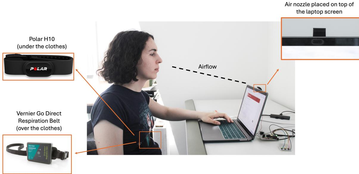
Fig. 6. The study apparatus includes the *BreathePulse* device that blows a subtle airflow to guide slow breathing. The air nozzle is placed on top of the laptop screen and directs the airflow to the participant's nostrils. Participants wear the Vernier Go Direct Respiration Belt around the chest to collect the respiratory rate. Participant also wears the Polar H10 heart rate monitor under the clothes to collect the ECG.
