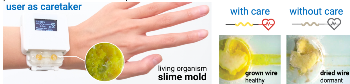
FIGURE 1. This example depicts a design centered around the user as a caretaker . This smartwatch has a slime mold in its circuitry. Its design requires the user to care for the organism (by feeding and watering the integrated living organism). Without care, the organism will dry up and stop functioning as a wire for the smartwatch, disabling its heart rate sensor.
