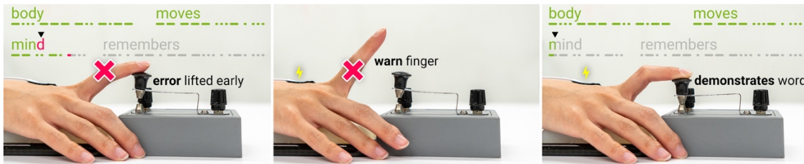
Figure 6: Adaptive-EMS applied to learning a sequence of button presses, such as in Morse code. In this example, the entire the word “mind” is played back when the user makes a mistake only in the final letter, this provides more context for the adaptive-correction.
