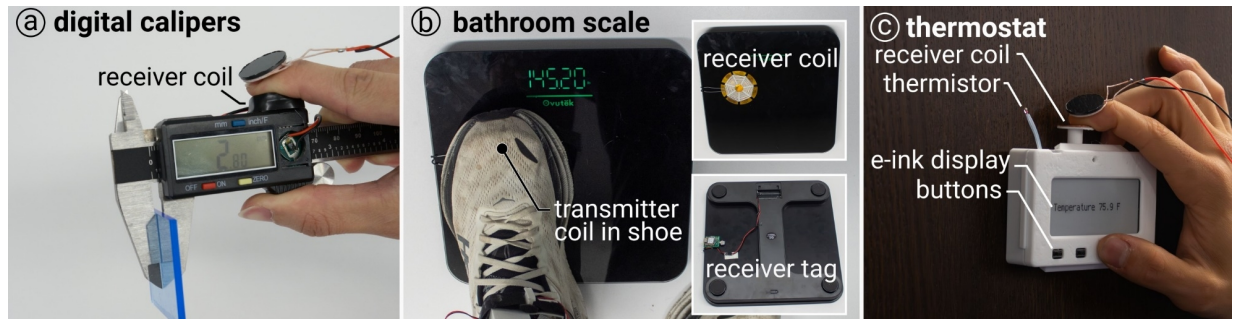
Figure 15: (a) A digital caliper is powered while the user holds it. (b) A digital body scale is powered on when the user, wearing shoes embedded with transmitter coil, steps on it. (c) A batteryless thermostat that contains an ink display and a thermistor.
