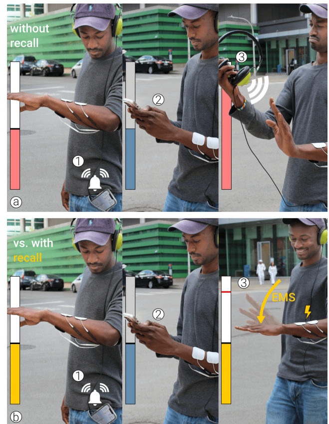
Figure 3: Illustrating the recall technique using an embodied slider for eyes-free volume control (via wrist).
